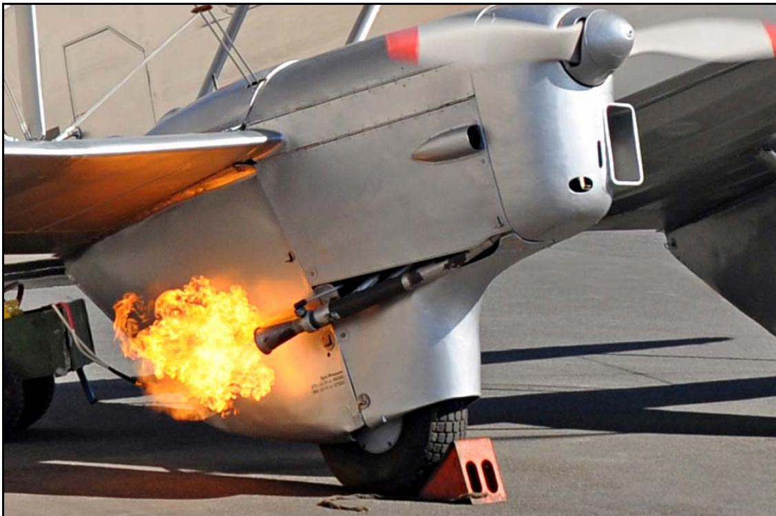
A secondary risk is that of igniting an explosive air/fuel mixture within the rear engine cowlings, due to spillage during refuelling or venting of a full tank when the fuel expands with temperature. Accumulated dry grass cuttings add obvious potential for combustion.
