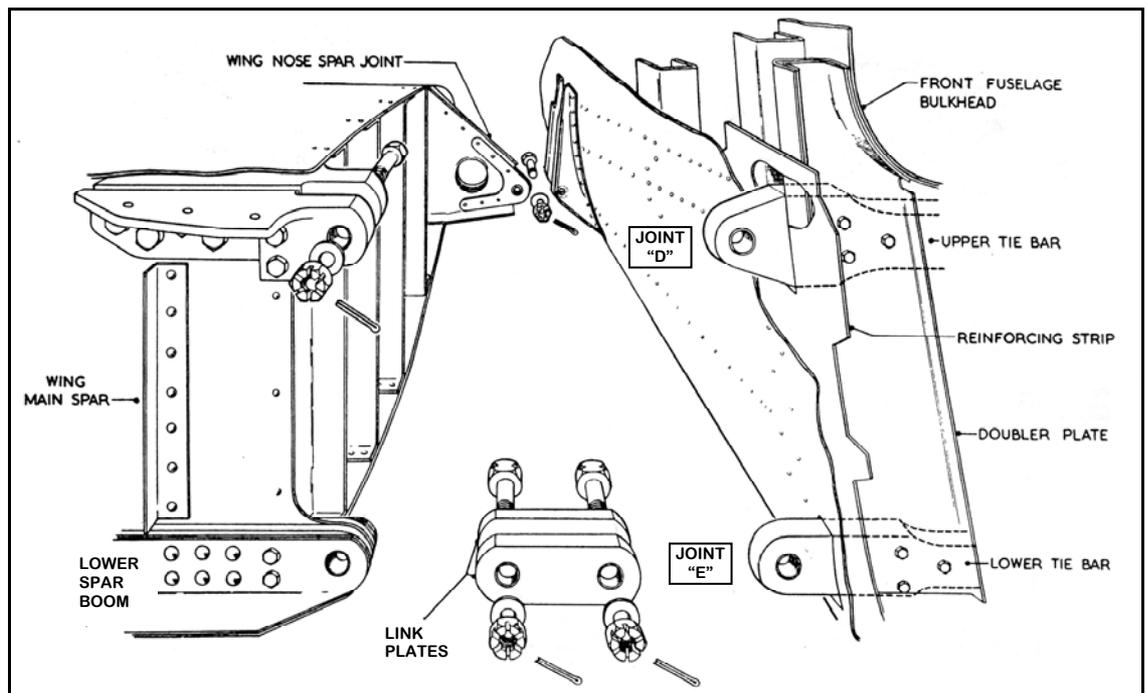
**FIG. 1. CONFIGURATION OF WING-TO-FUSELAGE SPAR ATTACHMENTS**
